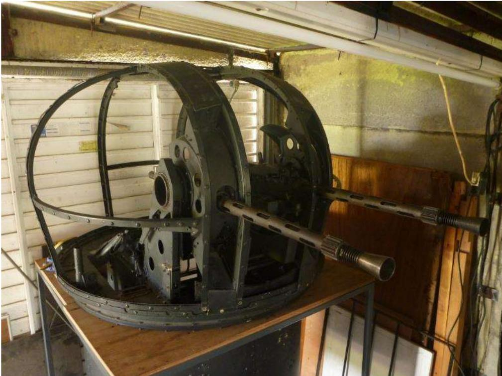
Below is a gunner's view of the guns with the face armour and control panel between them and the control handles to the outboard rear.
